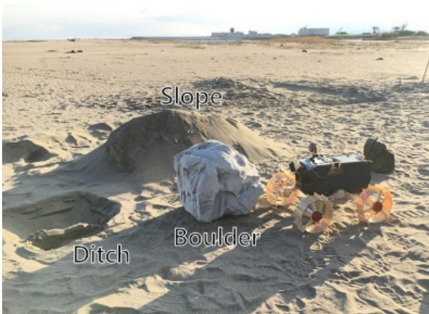
Fig. 11. Overview of the emergency stop algorithm trial experiment at Sendai beach.
